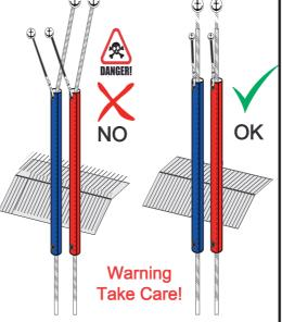
When securing to a structure ensure that the the path of the rope is not deviated by the protector -because thi would cause the Velcro to be pulled open when the rope is loaded
