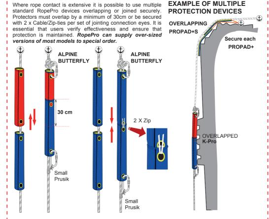
Where edges are more severe and rigging can not achieve clearance it is possible to 'Wrap' or 'Stack' RopePro devices to provide multiple layers of devices.
