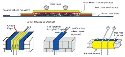
The ProPad+ can be used open or closed depending on application and stability of the loaded ropes. When closed – all connection eyes align to allow full through connection using karabiners or threaded rope. Can be secured direct to beams and other mid-rope obstacles - use 6mm -11mm rope
