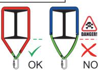
**Protect Nylon Slings** from structural damage
