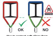
Use to protect soft slings from steelwork damage
