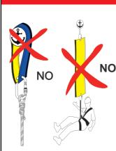
Never use to support any load - Never connect both ends for use as an anchor!
